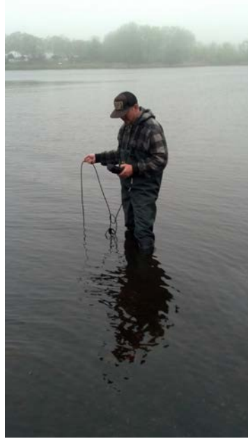
Photo 3: Water Quality Monitoring was performed using handheld YSI multi-probed sonde supplied by the NJDEP. Photo taken in 2014 during Sampling Event 1.
